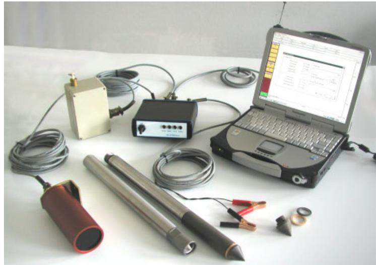
Above: Complete CPT-equipment from Geotech - probe, depth encoder, HC-system, interface box, laptop.
